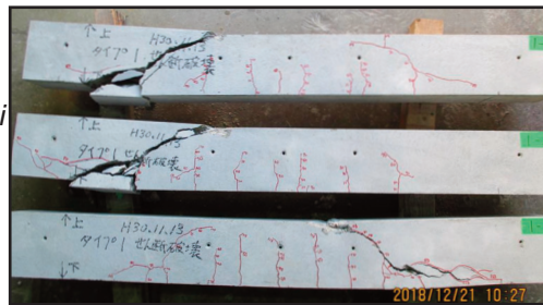
Figure 15: Variation of crack propagation in a concrete beam test (Dr. Mao Kurumatani)
