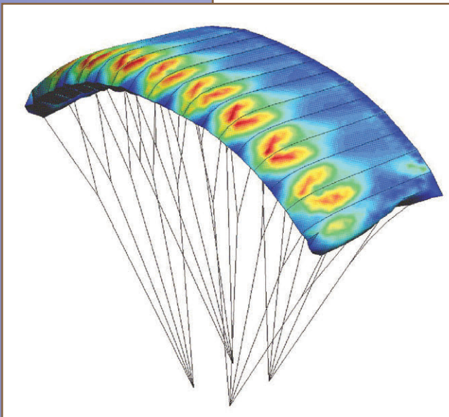
Figure 3: FE analysis of a parachute, modeled with 3-noded membrane triangles. This is Fig. 8.48 taken from the book
