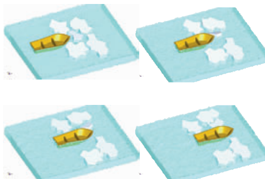
Figure 9: 3D PFEM simulation of a boat colliding with five ice blocks
