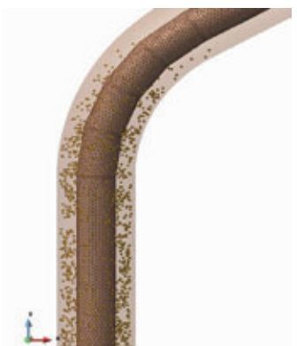
Figure 12: Transport of drill cuttings in mud within a curved borehole pipe with rotational annulus
