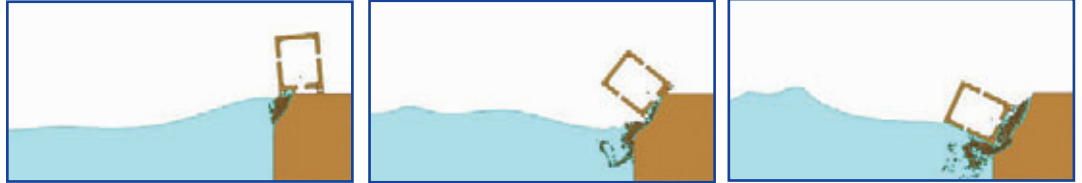
Figure 5: Erosion of a soil mass due to sea waves and falling into the sea of an adjacent lorry
