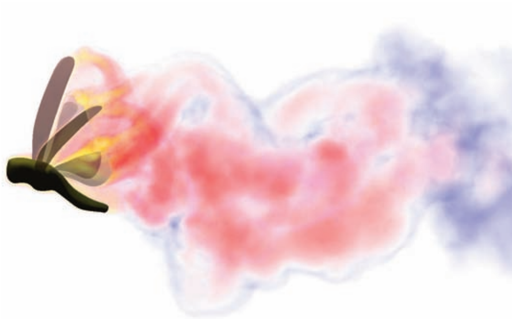
Figure 7: Vorticity magnitude at an instant during the flapping cycle
