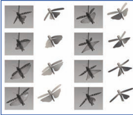
Figure 4: Comparison of computational model and wind tunnel pictures at eight points in time. Viewing angles are matched approximately. Wind tunnel pictures courtesy of Gabbiani and Chan
