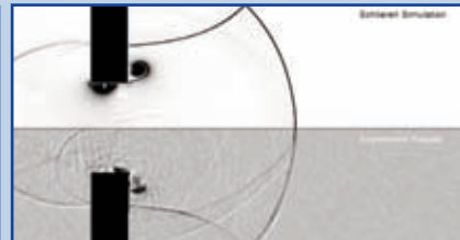
Figure 4: Figure taken from the lecture of Shachar Berger at ISCM-31, showing the comparison between numerical and experimental schlieren images of a shock wave
