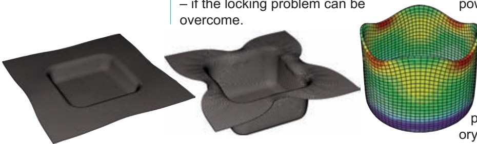
Figure 7: Forming results computed by means of Q1STs
