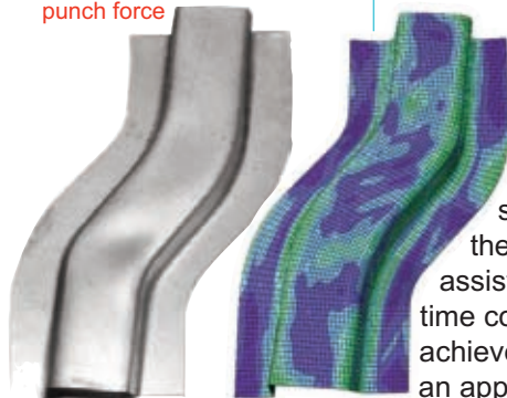
Figure 2: Springback of an S-rail
