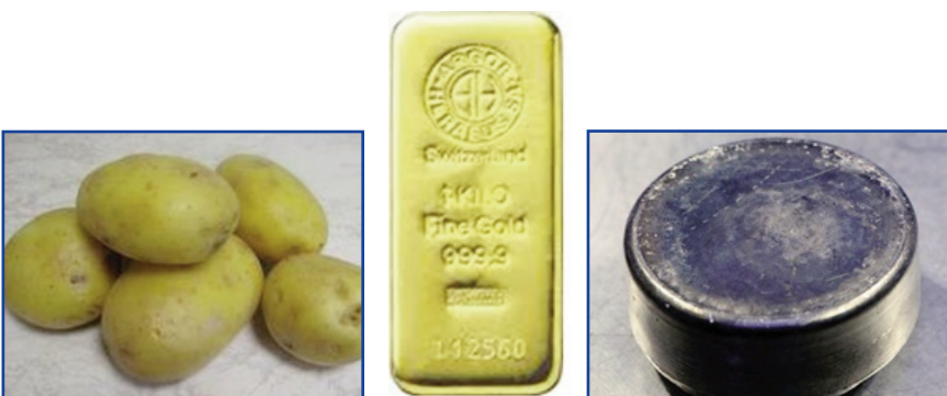
Figure 1: 1.0 kg of potatoes, 1.000 kg of gold and 1.00000 kg of plutonium. Same weight?
