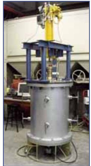
Figure 3: UNSW suction controlled calibration chamber
