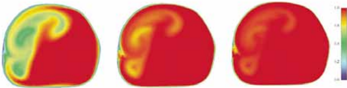
Figure 4: Spatial concentration of nanoparticles for different non-dimensional mass transfer coefficients (from left to right: Sc = 10, 100 and 500 ).
