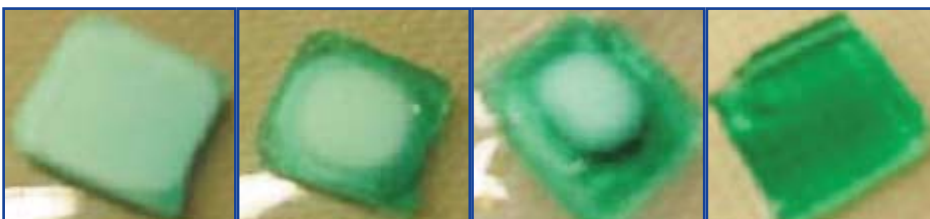
Figure 3: Sequence of images showing a collapsed to swelled transition in a hydrogel specimen.
