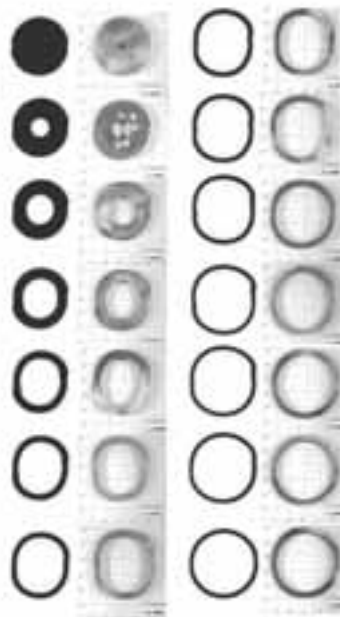
Figure 5: Section through the rolls. The color map indicates the equivalent plastic strain and the dots the mapped data.
