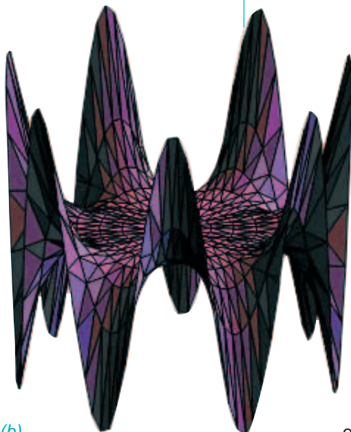
(b) solution obtained for a problem defined on a circular domain with exact solution as a seventh order polynomial. With 80 boundary nodes the accuracy achieved is 0.003 % in relative energy norm.
