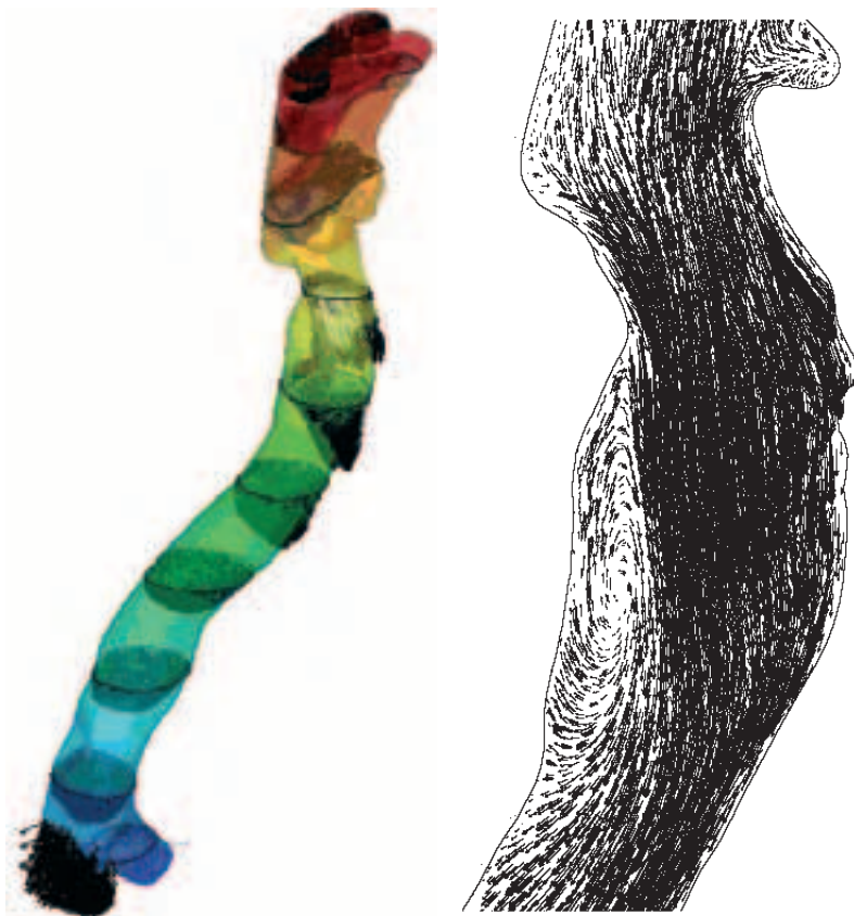
Figure 6: Velocity vector plots at an inhaling flow rate of 30l/m. Vectors (left) and recirculation below vocal cords (right)
