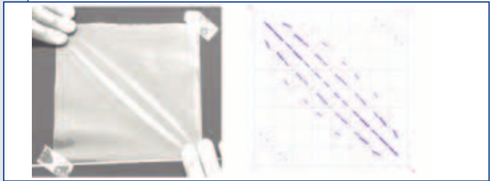
Figure 5: Wrinkles in a membrane - comparison of computational results and a "qualitative experiment"; from a presentation of Zelkha, Gal and Levy.
