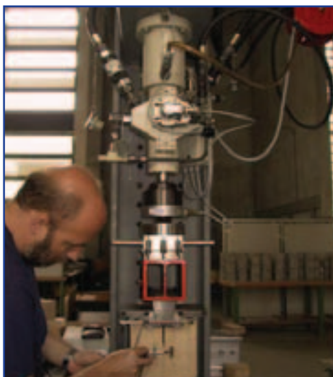
Figure 5: Wedge splitting test performed on a small specimen (courtesy of V. Saouma)
