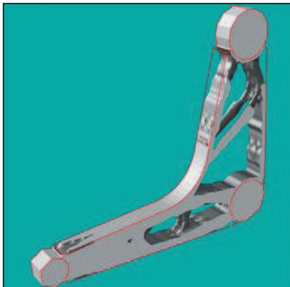
Figure 1: Optimization of a car suspension triangle by topological optimization (courtesy of F. Jouve)
