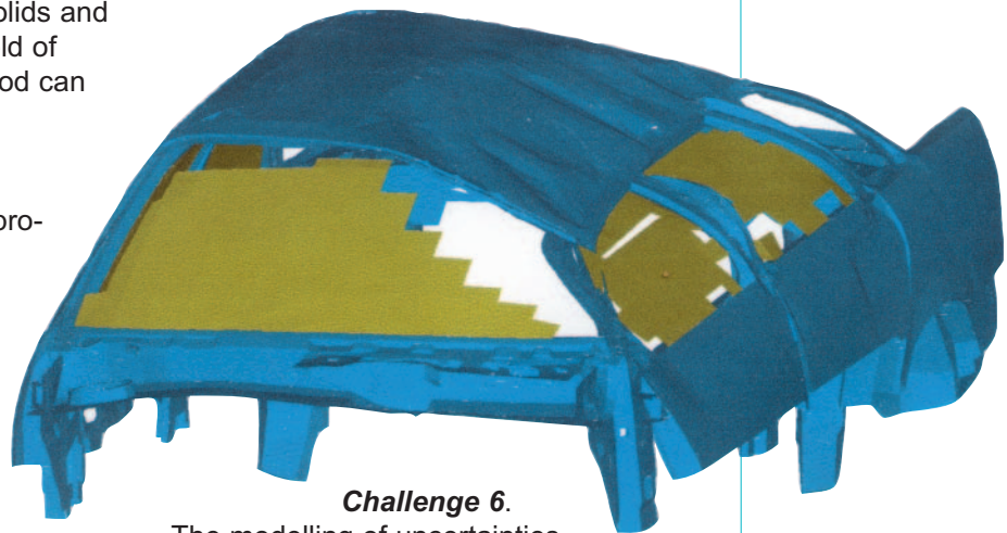
Figure 3: Crushing of a motor car model
