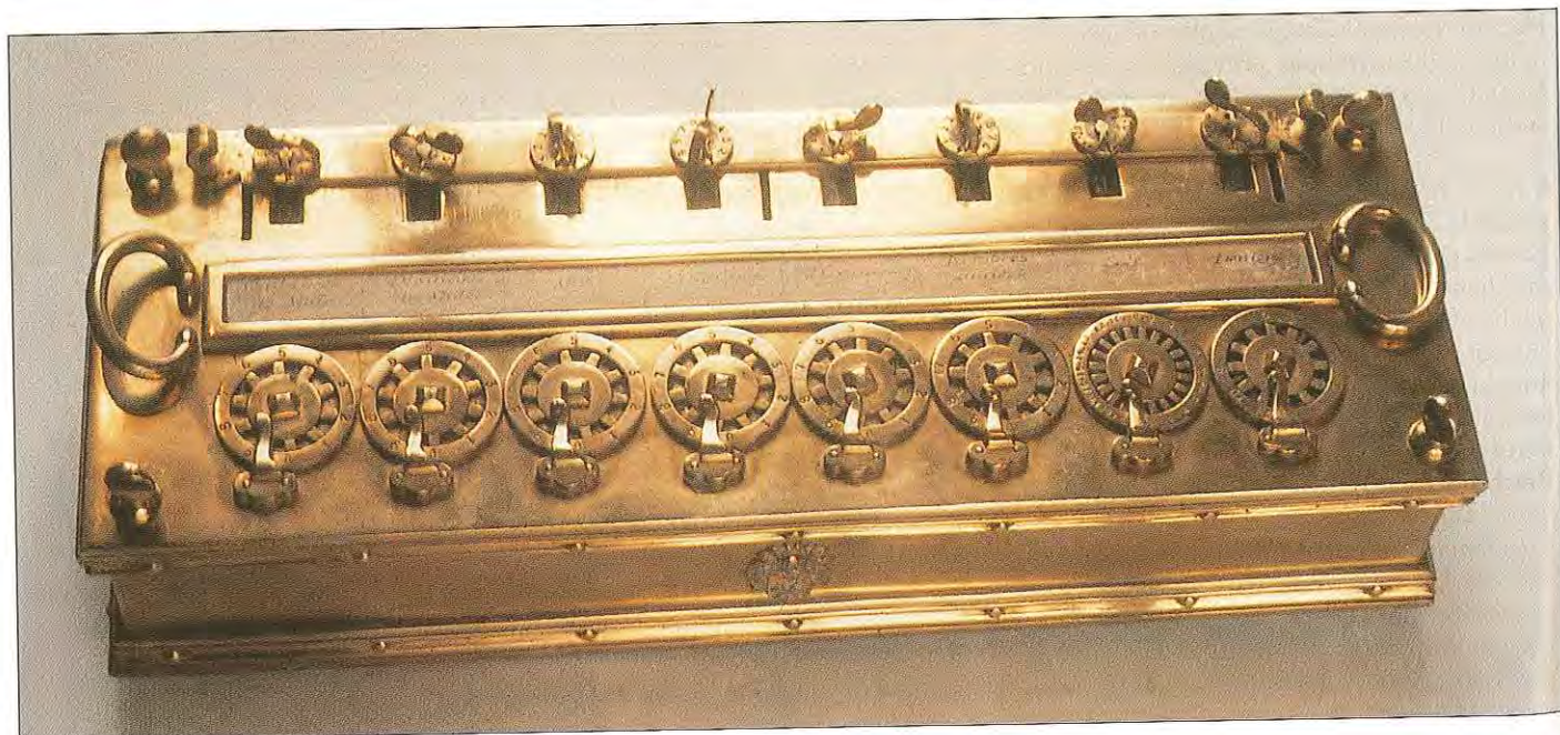
Figure 7: Pascal's calculating machine for adding and subtraction from 1644
