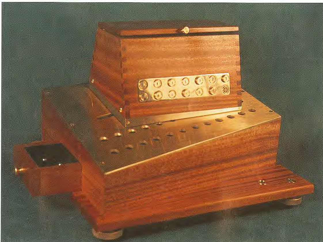
Figure 11: Model of a binary calculating machine (for adding and multiplication) according to Leibniz's ideas in his manuscript De Progressione Dyadica , 1679, reconstructed by L. v. Mackensen, Landesmuseum Kassel.
